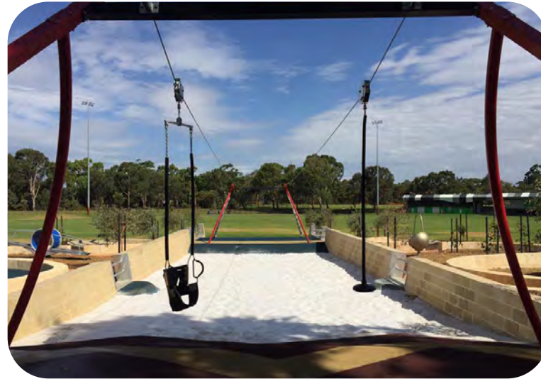
Above: Inclusive flying fox (dual ride) with harness seat and pommel seat
