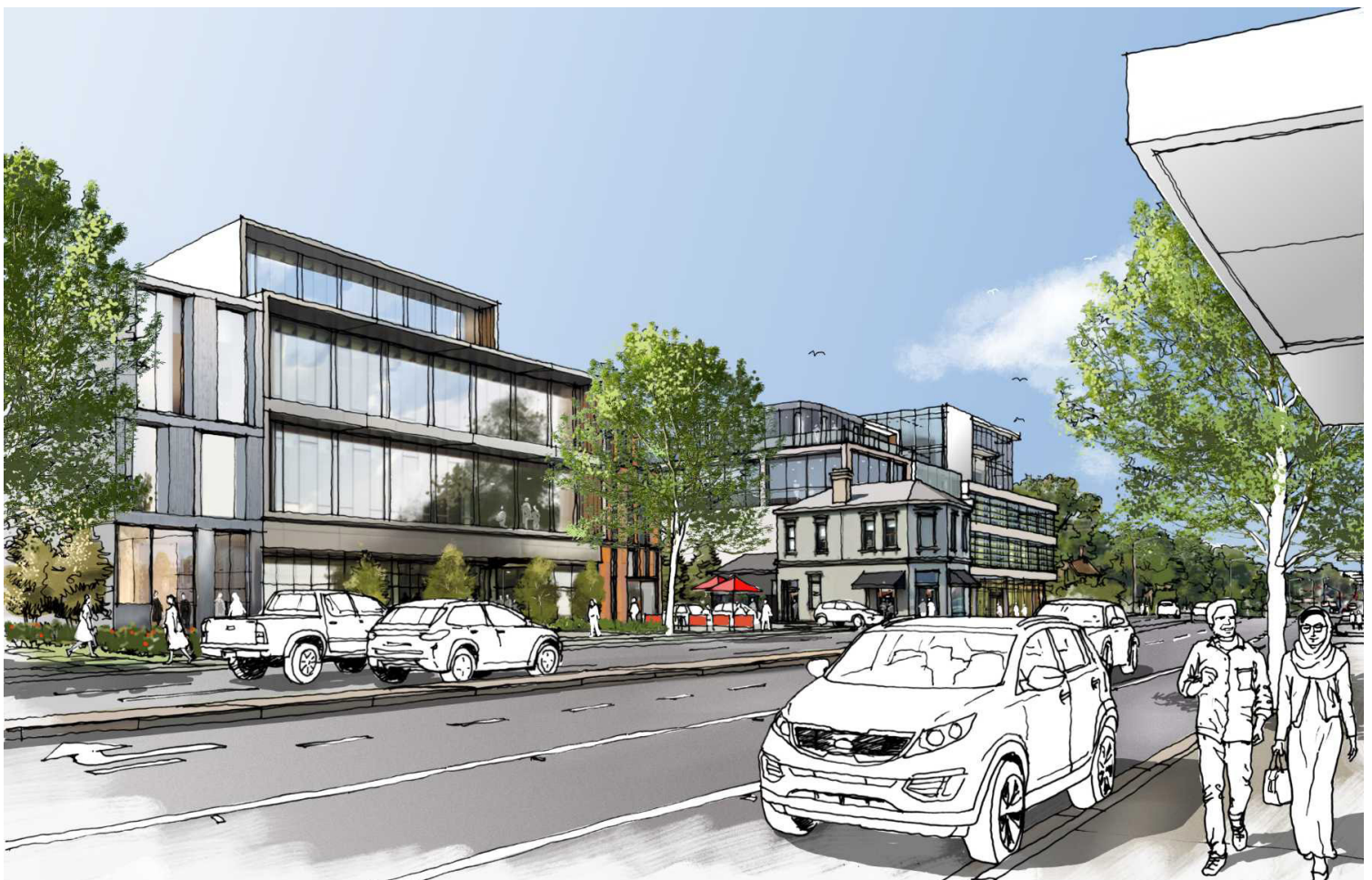
Illustration depicting maximum building and street wall heights for development in Precinct 2 on Heidelberg Road as proposed by design guidance.
