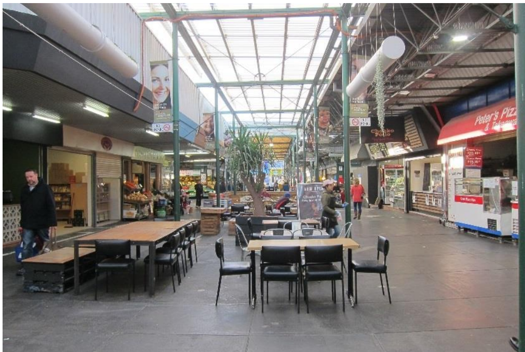
Figure 23. Image shows Shed 2 on the left and Shed 5 on the right. Space frame structure still evident on Shed 5 but not on Shed 2. Tent-like walkway canopy has been replaced with clear flat covering in this location. (Source: Context 2017).
