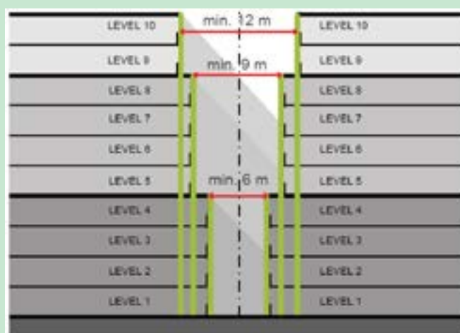
Figure 23. Building separation requirements for secondary outlook
